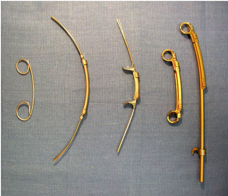
FIGURE 6.1 Evolution of the Vertical Expandable Prosthetic Titanium Rib (VEPTR) showing versions from 1987, 1989, 1991, and 1996. (The rightmost item shows the device in its expanded mode, to its left is the unexpanded device.) (Courtesy of Robert M. Campbell, M.D.)
