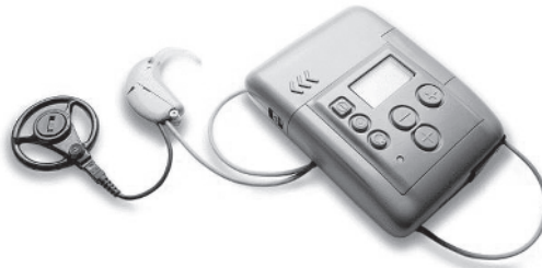
FIGURE F.2 Body-worn processor. (Courtesy of Cochlear Americas Corporation.)
