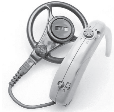
FIGURE F.1 Ear-level processor. (Courtesy of Cochlear Americas Corporation.)
